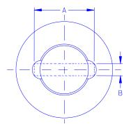
Figure 3: Retainer Removal Tool Dimensions
