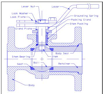
Figure 2: Typical One Piece Valve Assembly
