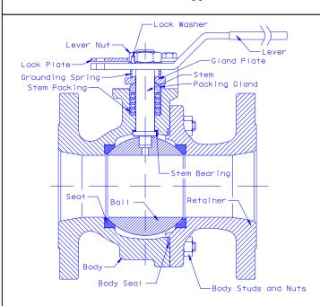
Figure 1: Typical Standard Port Valve Assembly
